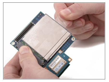
Grasp the wireless interface board with one hand and the clear plastic tab on the Airport card with the other hand, and pull the Airport card from its connector.
