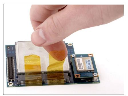
• Remove the yellow tape securing the Airport card to the wireless interface board.
