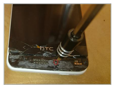
Use your T6 Torx screwdriver to remove the single screw that holds the body to the aluminium back
