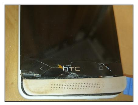
Use a plastic opening tool to remove the bottom speaker cover
