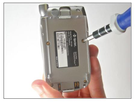
• Unscrew the four screws behind the battery
