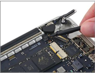
Use the flat end of a spudger to disconnect the keyboard backlight cable and move it out of the way.
