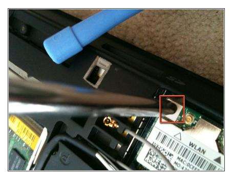
remove the one and only philips screw securing the WiFi card in place.
