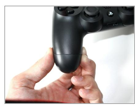
Remove the bottom half of the controller while monitoring the triggers and springs within.
