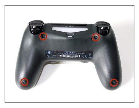
Remove the four Phillips #00 screws from the back of the controller.
