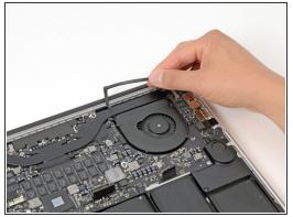
In the same manner described above, release the adhesive and flip back the heat sink cover on the left fan.
