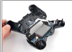
• Flip the rear case over the top of the controller and lay it down, being careful not to strain the interconnect cable.
