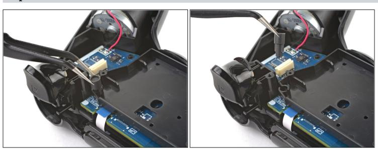
• Grab and remove the reset button extension from its recess in the battery bracket.
