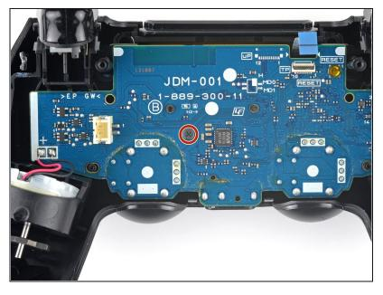
• Use your Phillips screwdriver to remove the 6.4 mm screw securing the motherboard.
