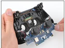
⚠ Be careful not to strain the vibration motor cables. Follow this guide to re-solder the vibration motors if they break off the motherboard.
