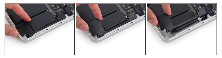
• Lift the corner of the left speaker up and slide it out around the battery to remove it from the upper case.
