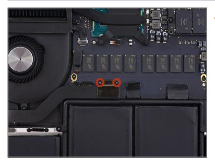
Remove the two 2.1 mm T5 Torx screws securing the logic board end of the I/O board cable bracket.
