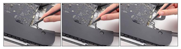
• Use a spudger to pry each of the four antenna connectors straight up off their sockets on the AirPort/Bluetooth card.
