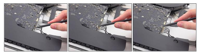
(i) If necessary, use the tip of a spudger to peel back the tabs covering the antenna connectors.
