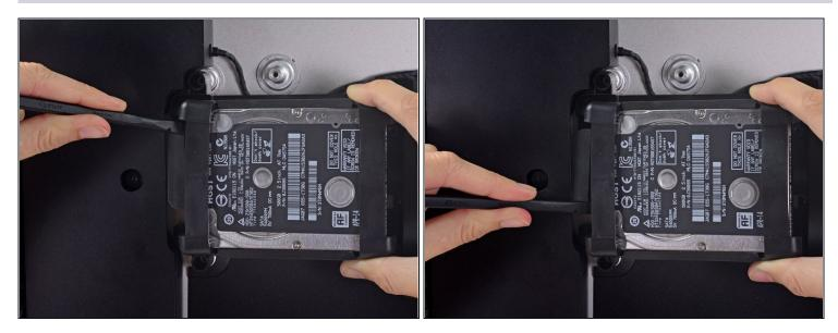
• Use a spudger to disconnect the single SATA power and data combo cable by gently prying its large plastic connector away from the hard drive.
