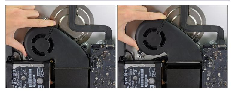
• Lift and remove the fan from the iMac.
