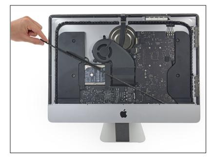
• Remove the lower support bracket from the iMac enclosure.
