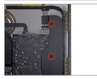
• Remove the two 10.0 mm T10 screws securing the right speaker to the rear enclosure.
