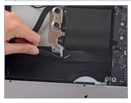
• Use a pair of tweezers to peel the tape covering the exhaust duct.
