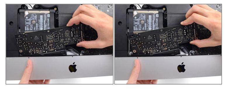
• Slide the power supply to the right to clear the screw posts on the rear enclosure.
