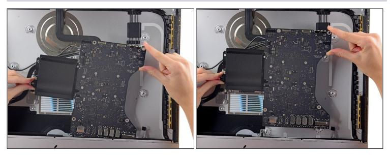
• Lift the logic board straight up and out of the iMac.
