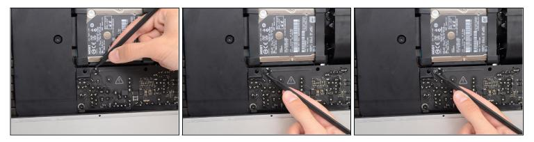
The next few steps bring your hands close to the exposed face of the power supply. **Do not** touch the face of the power supply or any of the exposed solder. Touching it risks a high voltage shock from the many large capacitors attached to the board.
