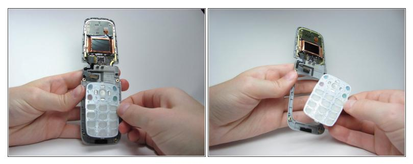
• Remove the keypad from the phone by lifting the keypad off the phone.
