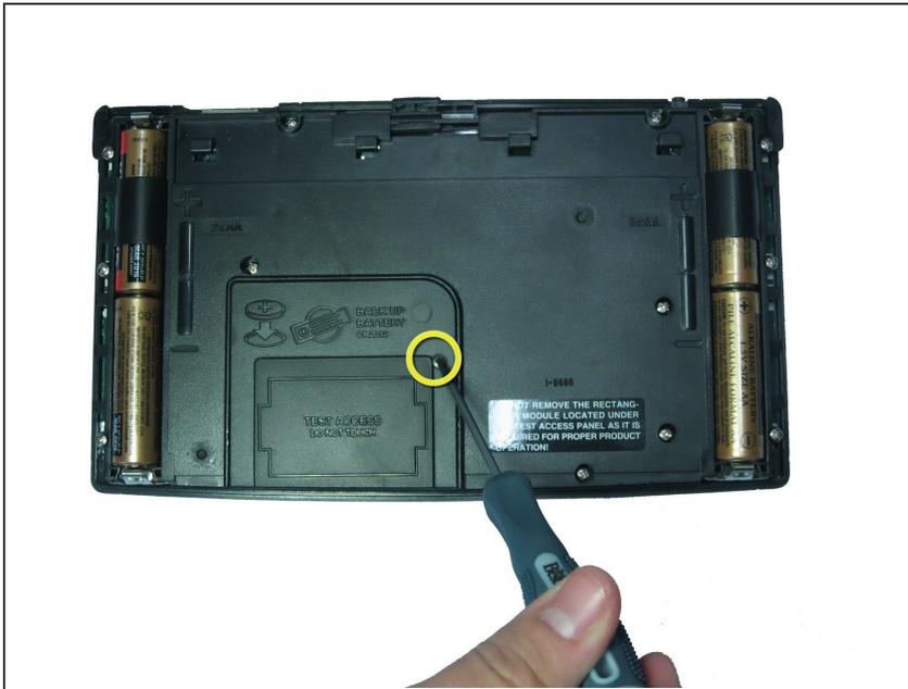
**!** Before removing the backup battery make sure your AA batteries are installed so that there is no loss of information.
