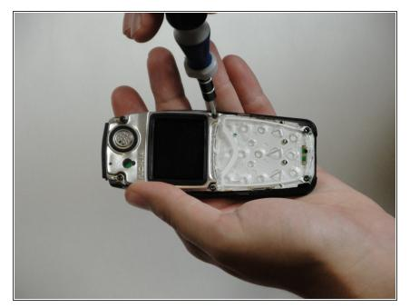
Unscrew the six screws with a Torx screwdriver (six-pointed star shaped bit).
