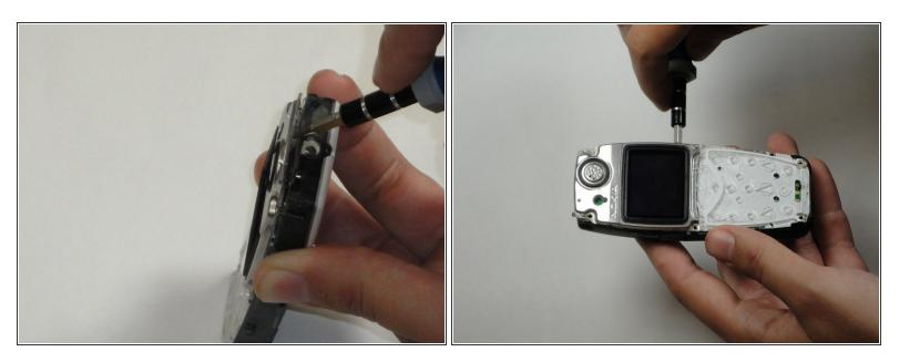
• Insert a flat screwdriver between the black body and plastic layer.
