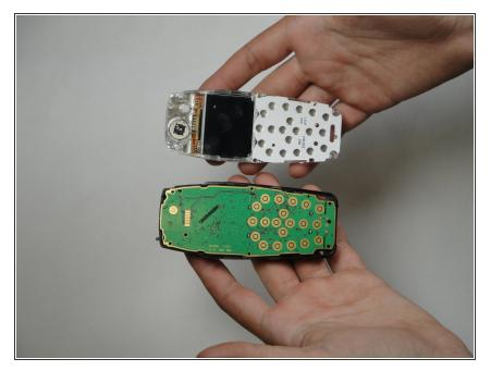
• Pry the layers apart. The LCD and plastic layer will lift out as one piece.
