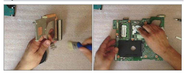
• Clean the old thermal paste / compose from the CPU.
