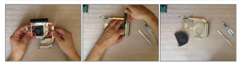
• Disassemble the Heat Sink system to clean the fan and the radiator from inside.
