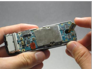
Use the iFixit opening tool to remove the yellow tab on the motherboard.
