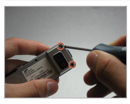
Remove the two 7.3 mm screws from the camera and the speaker at the bottom back plate of the phone using a Phillips #00 screwdriver.
