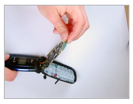
Lift the motherboard from the bottom to loosen it.
