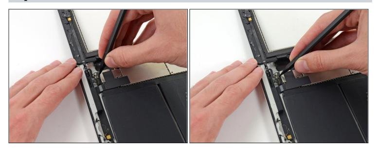
• Flip up the retaining flap on the home button ribbon cable ZIF connector.
