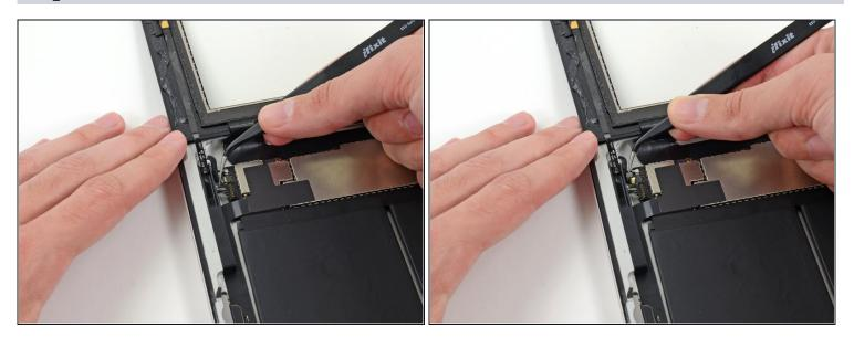
• Use a pair of tweezers to pull the home button ribbon cable straight out of its socket on the logic board.
