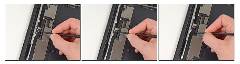
• Flip up the retaining flap on **both** of the digitizer ribbon cable ZIF connectors.
