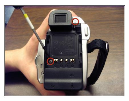
Remove the two screws connecting the back plate to the camera base.
