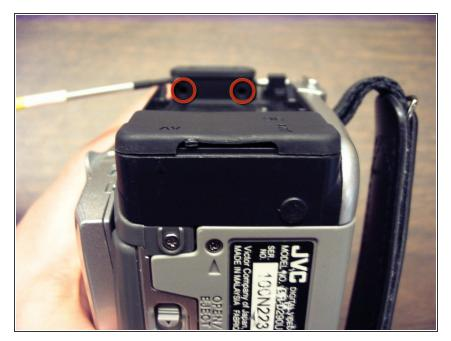
Remove the two screws on the underside of the camera eyepiece.
