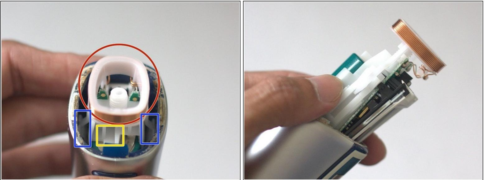
**!** Do not pull the coil ring as the wire will break away from the the circuit board
