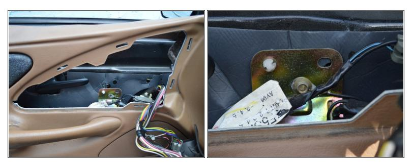
Remove the bolt holding on the plastic to the door.
