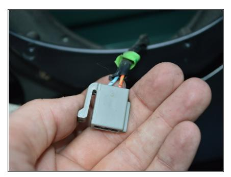
Once you've removed the speaker off of the door by removing the bolts unplug it. This is the connector
