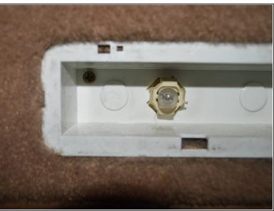
Pry the plastic off of the light enclosure on the bottom of the door. Once you remove it, take the screw out. This is the only other screw holding the door on.
