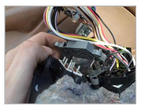
Begin romving the power windows connector by removing the screws, then prying off the plastic connectors
