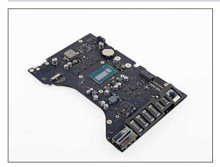
During reassembly of the logic board, pay attention to the position of the I/O connectors. When the board is back in the case, insert a USB or Thunderbolt cable into one of the connectors to align it perfectly.
