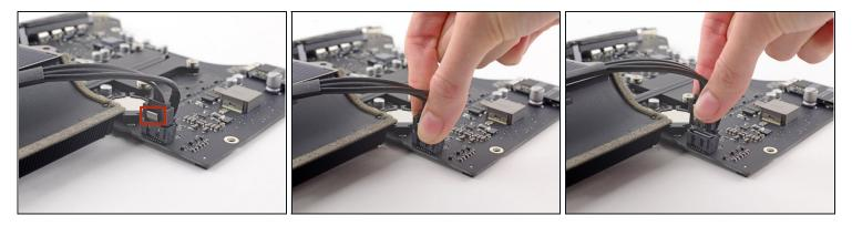
(i) The SATA data connector has a clip that must be pressed to allow removal.
