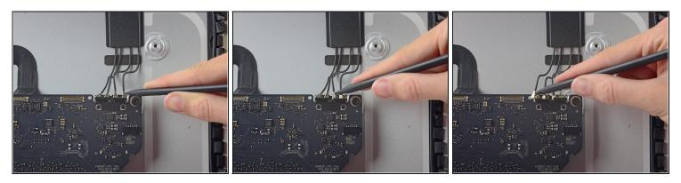
• Use the tip of a spudger to disconnect each of the four antenna connectors from the AirPort/Bluetooth card.
