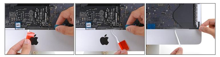
• Peel away the white backing behind the strip to expose the remaining adhesive.
