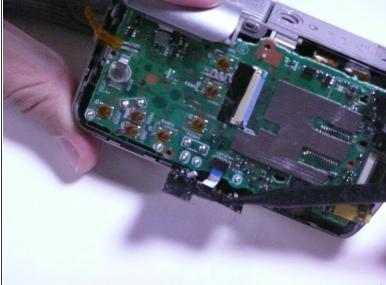
Remove black sticky tape from circuit board and camera case.
