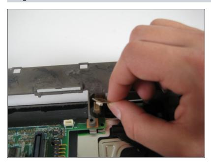
Disconnect the power connector from the motherboard.
