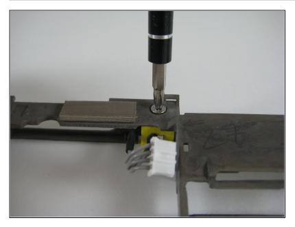
Remove the screw and pull the plug out from underneath the metal frame.
