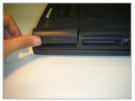
• To remove the battery cover, use your hands to slide it upwards.
