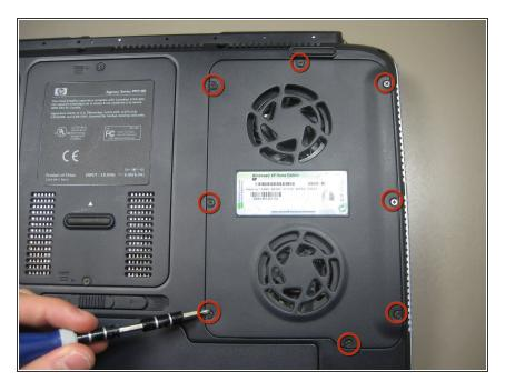
Loosen the eight Phillips screws around the plate to remove it.
