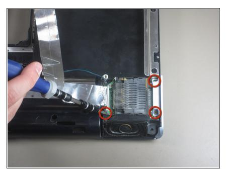
Remove the 3 screws connecting the spearker.
