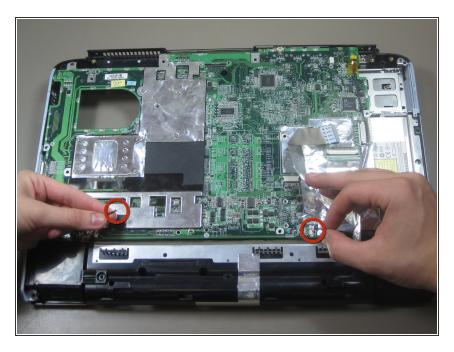
Disconnect the speaker cables from the motherboard.
