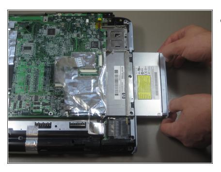
Slide out the optical drive if it wasn't removed in Step 9.
