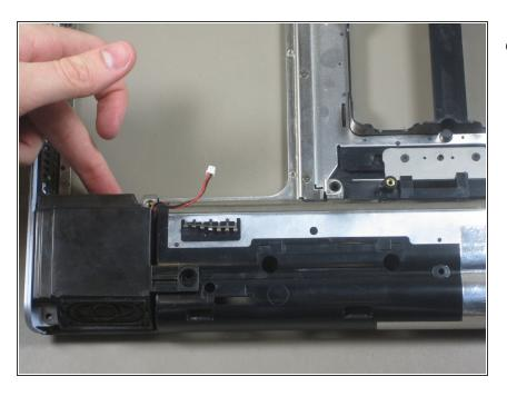
To remove the second speaker simply lift it up and out.
