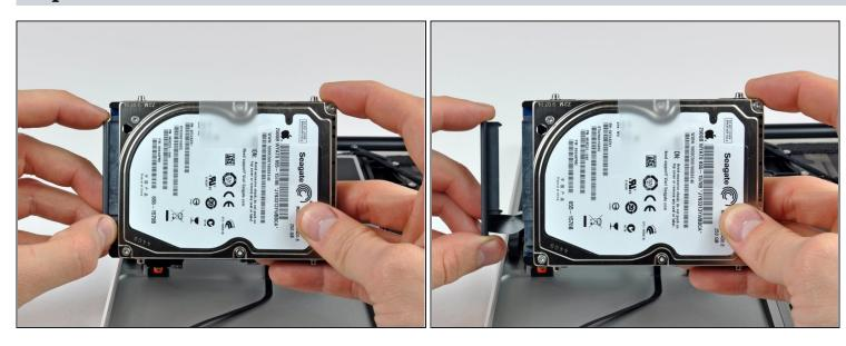
• Remove the hard drive from its cable by pulling the cable connector straight away from the drive.
