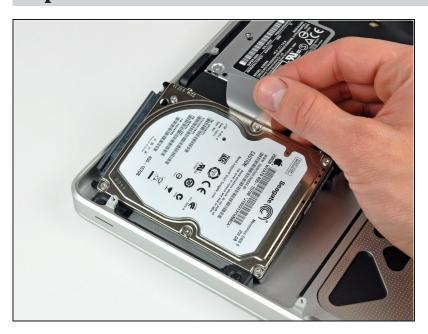
Lift the hard drive out of the upper case by its plastic pull tab, minding the cable attaching it to the computer.
