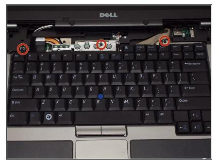
Locate the three philips head screws above the keyboard. One is above the 'Pause/Break' key; one above the F7 key and one above the 'Esc' key. Remove all three.
