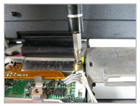
Remove a single screw from the metal plate that secures the display cable.
