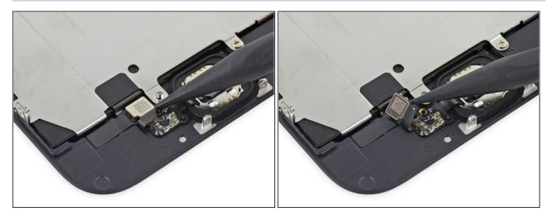
• Use the point of a spudger to disconnect the home button cable connector by pushing it up and away from the home button.
