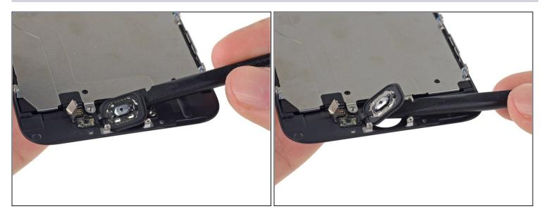
• Peel the home button the rest of the way off of the display by prying gently with a spudger.
