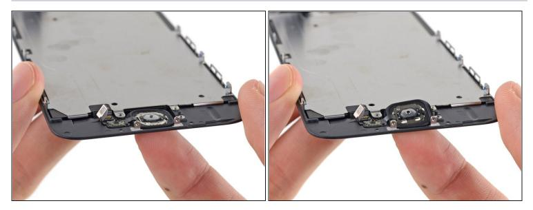
A The rubber membrane surrounding the home button is very thin and tears easily.
