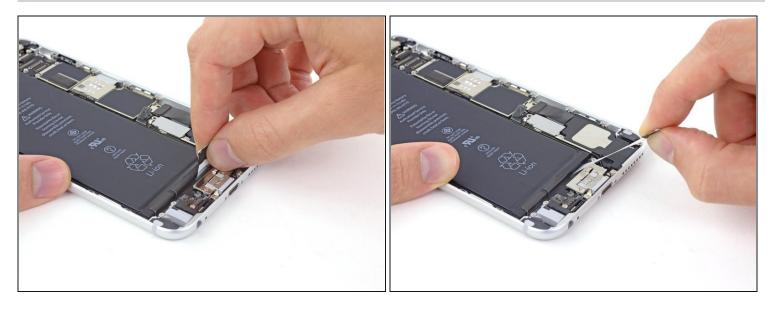
Try to keep the strips flat and unwrinkled during this procedure; wrinkled strips will stick together and break instead of pulling out cleanly.
