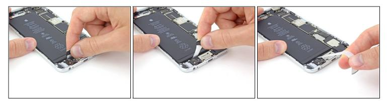
• Peel back the final battery adhesive tab from the bottom edge of the battery. Gently pull the battery adhesive tab upward and away from the battery, allowing the adhesive strip to slowly slide out from between the battery and the rear case.
