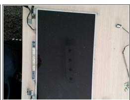
• remove all the other screws and henges, so you can remove the lcd screen from the frame.
