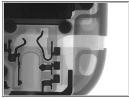
The iPhone 6 has the antennae clearly separated in the design of its case. An aesthetic feature loved by some, hated by others. Here it is seen from the inside out, both left and right of the phone. Also seen here is the TouchID sensor and the Lighting data and power connector.
