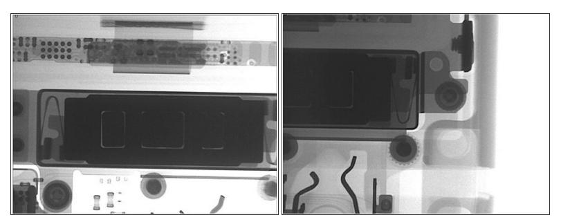
• It is well known Apple likes to play with the vibration motor in the iPhone products. The iPhone 4 used a counterweight design, the iPhone 4S a linear oscillator, the iPhone 5/5S went back to a counterweight design. For the iPhone 6 it seems we're back to the linear oscillator idea.
