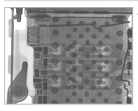
The SIM card connector is well defined in the iPhone 6. Note the voiding in the solder balls of the connector.
