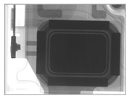
Although the speaker assembly channel assembly changed in the iPhone 6, it seems Apple is still using the same speaker as used in the iPhone 5S.
