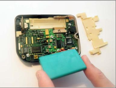
• Remove the rubber placement pad that sits under the battery and set aside for later use. Gently fold back the battery, making sure the small plug connecting the battery to the logic board remains intact. Extra care should be taken as this part is quite delicate and easy to damage.
