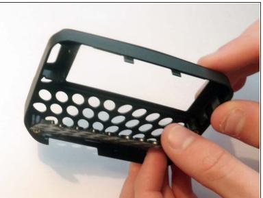
Flip the newly separated front portion of the casing over so that the front of the device is facing upwards, causing the keypad to fall loose.
