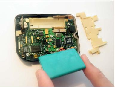
• Remove the rubber placement pad that sits under the battery and set aside for later use. Gently fold back the battery, making sure the small plug connecting the battery to the logic board remains intact. Extra care should be taken as this part is quite delicate and easy to damage.
