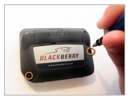
Use a T9 Screwdriver to unscrew the two screws on the backside of the BlackBerry, one on the bottom left and one on the top right.
