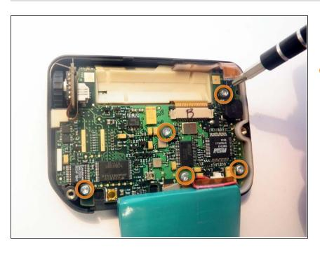
Use the T9 Screwdriver to remove the five visible screws: Top right, bottom right, middle center, bottom center, bottom left.
