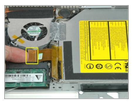
Disconnect the orange optical drive ribbon cable from the logic board.
