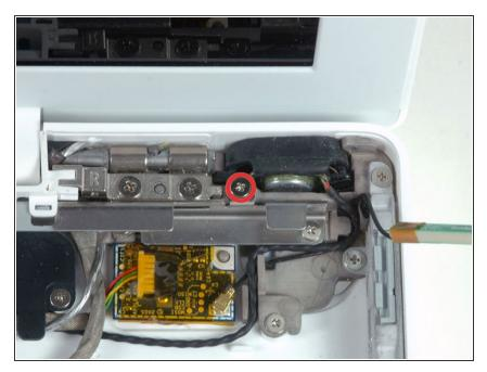
Remove the single Phillips screw securing the right speaker to the lower case.
