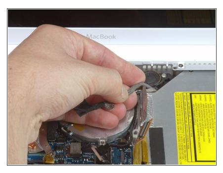
Pull up the display data cable from along the edge of the optical drive to reveal a silver Phillips screw.
