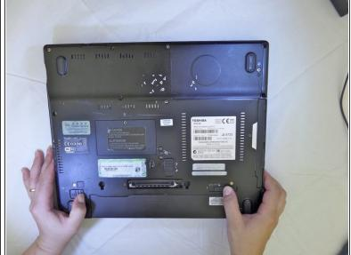
Slide both tabs outward at the same time to release battery pack.
