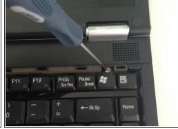
Using a #00 phillips head screwdriver, remove the two 4mm screws found underneath the keyboard strip.
