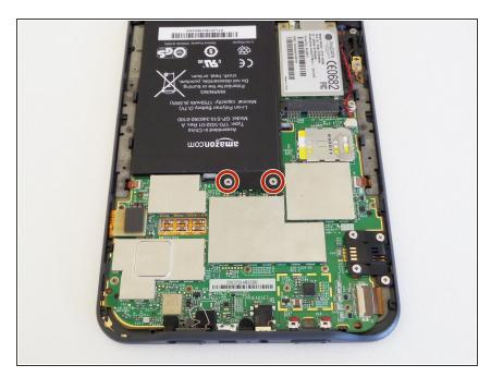
Unscrew the two silver 4 mm Phillips screws securing the battery connector.
