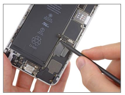
Use the tip of a spudger to disconnect the interconnect antenna cable from its socket on the logic board.
