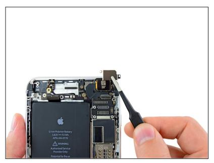
• Lift and remove the rear-facing camera bracket off the rear-facing camera.
