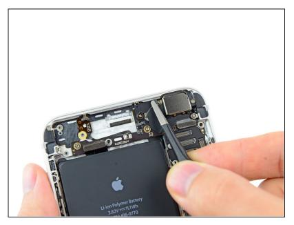
Use a pair of <u>tweezers</u> to peel back the piece of tape covering the hidden screw securing the rear-facing camera bracket to the rear case.
