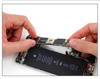
Carefully raise—but do **not** remove—the logic board,
