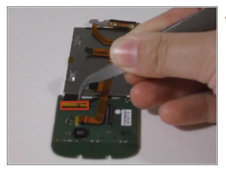
Pry the bar connecting the screen and circuit board by prying it gently upwards with tweezers to detach, separate, and remove the screen.
