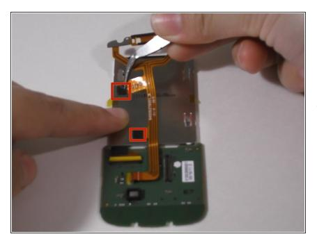
Lift the yellow strip away from the back of the screen by gently gripping with tweezers and
