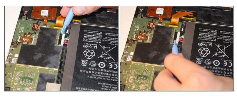
Using either the plastic opening tool or your fingers, gently pull on both sides of the plug to release
