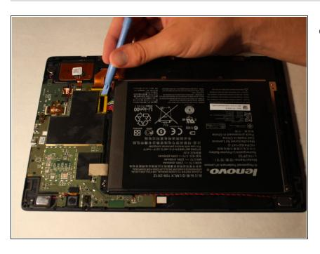
Pull off the plastic that is covering the battery cable.
