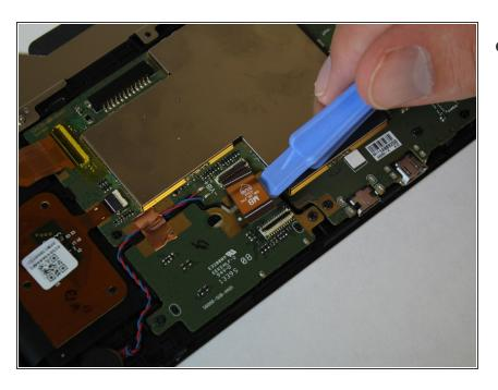
Flip the black tab up to unlock the cables by using the plastic opening tool.
