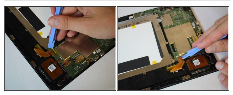
Remove the tape by pulling it up through the use of the plastic opening tool.
