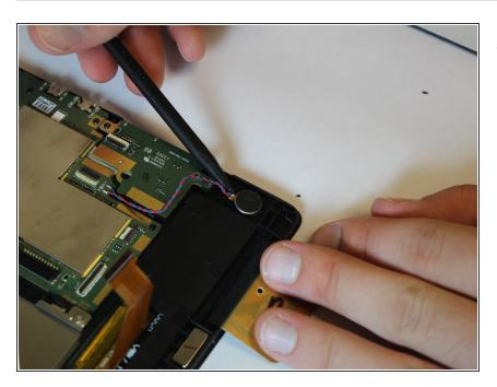
Use the spudger to pry up the vibration motor.
