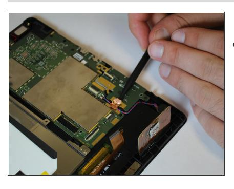
Lift up the cables connected to the tab by using the spudger tool.
