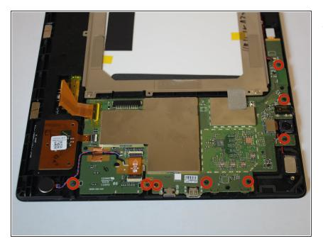
Remove the 3.16mm screws highlighted in red
