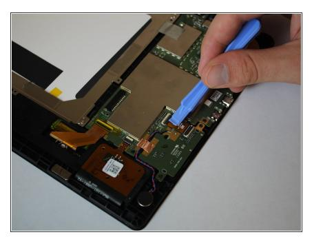
Force the ribbon cables out by pulling up the cables through the use of the plastic opening tool.
