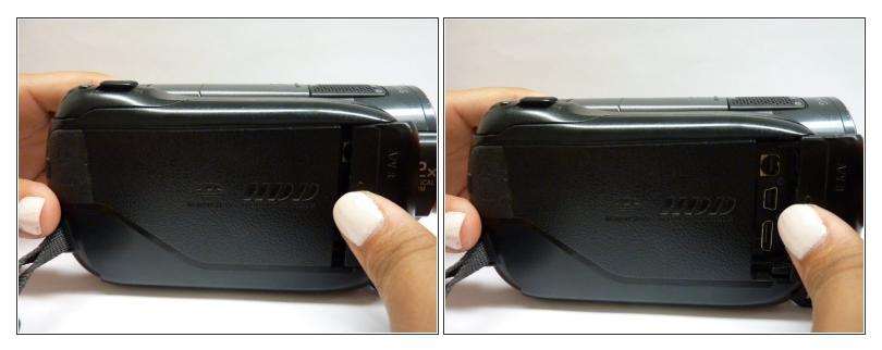
Open AVR –HDMI tab by sliding the flat panel next to the "HDD" engraving towards the camera's lens.
