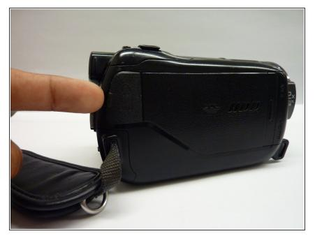
Using your nails, pry open the MIC tab so it points away from the camera. You'll feel a tongue-andgroove locking mechanism under the raised opening tab that needs to be pressed inward to release.
