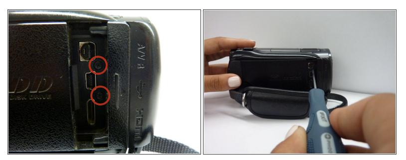
Under the AVR tab, on either side of the USB port and above the HDMI port, you will find two more screws. Remove them both.
