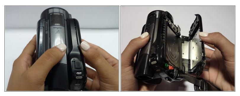
Hold the camera upright and, using your nail between the far right panel and the rest of the assembly, pry the hard drive open. If all screws were removed before this step, it should come away with very little effort.
