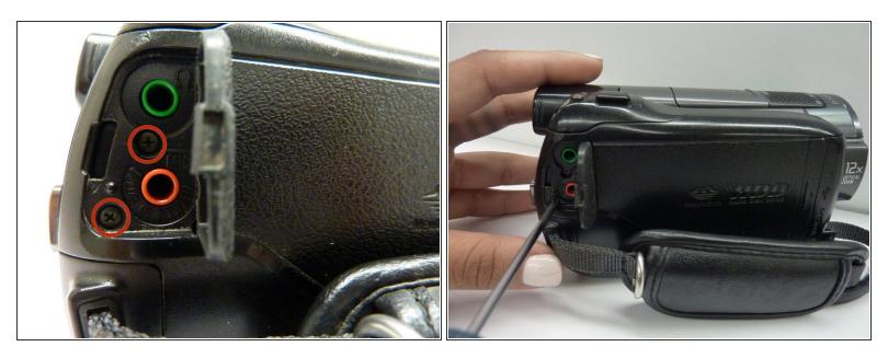
Under the MIC tab are two more Phillips-Head screws, one in between the red and green ports and one under the locking mechanism. Remove them both.
