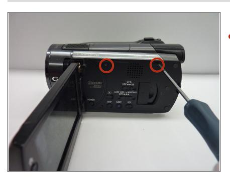
Remove the two screws on the control board.
