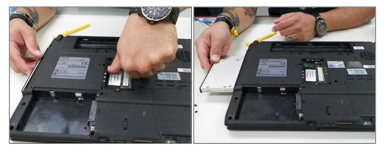
• Push down metal rod until optical drive pops out from its container on the side of the device.
