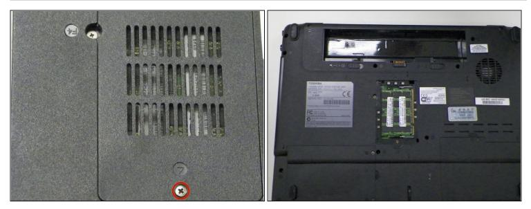
• Loosen **1** Phillips 4.2 mm size captive screw and lift cover off device to expose 2 RAM sticks.
