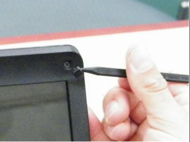
• Use tweezers to remove rubber screw covers on 4 corners of frame around screen.
