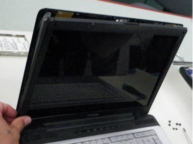
• Use flat side of spudger to pry the top and sides of the frame around screen.
