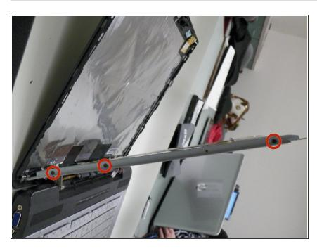
Remove 3 Phillips 3.2 mm screws from each side of the metal case around screen.
