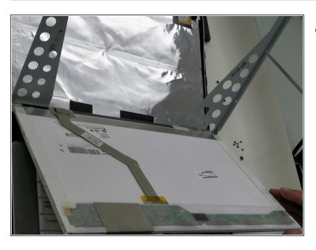
Pull the screen forward from the top out of the metal frame enough to see the back of the screen.
