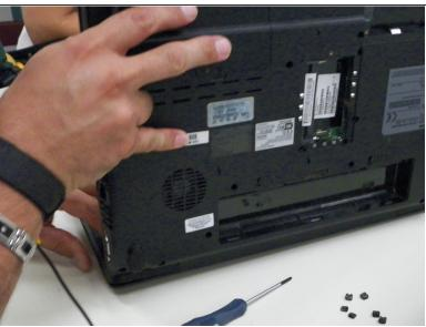
Turn device onto its screen side to access the bottom of hinge portion of the screen and push bottom piece of frame along device hinge until it loosens.
