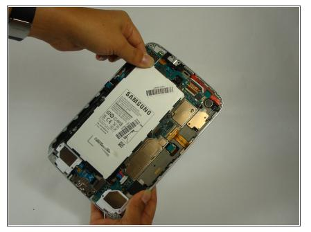
• Lift the top left corner of the battery up by the black tab.
