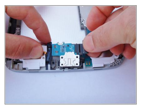
• Remove micro USB Port from its housing.
