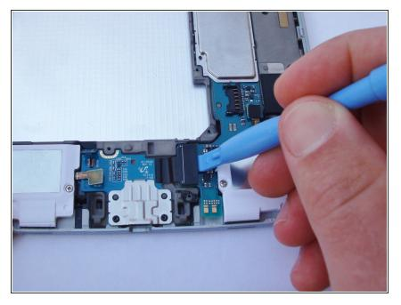
Gently lift up the large black connector on the right side of the component. This is the connector that was underneath the silver plate removed in the previous step.
