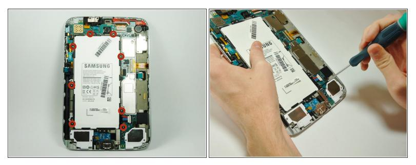
• Remove the 8 Phillips#00 3-mm screws holding the battery in place.
