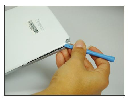
Using the plastic opening tool, start where the S-pen was located and carefully pry up the corner.
