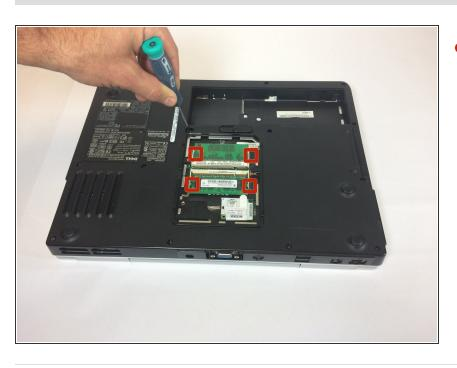
Pull the tabs located at red circles apart in order to separate the ram from its housing.
