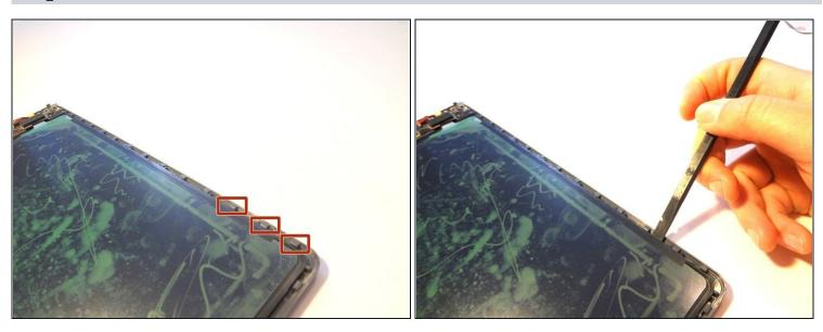
• Use a spudger (or gently bend the back plate of the device) to unsnap the snaps holding the screen in place.
