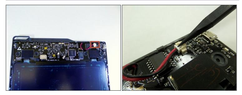
• With a spudger, press against the lip of the connector closest to the wires to remove the battery connector from the motherboard.
