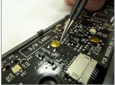
• Using <u>tweezers</u> gently go around the edges of the copper plate to remove the adhesive.
