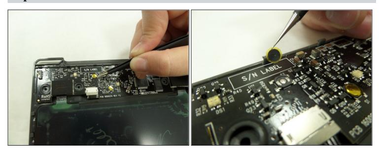
• Use tweezers to grip the outer edge of the copper plate and lift the button straight off.
