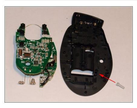
The circuit board is all one piece that lifts straight out. As you lift out the circuit board push the battery terminals so they clear the base plate. The reset pin will come loose after the circuit board is removed.
