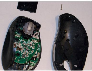
Remove the battery door and use a #8 Torx Tamper Proof Bit to remove the center screw. Pry the cover of the mouse starting from the back and lifting it up toward the wheel.
