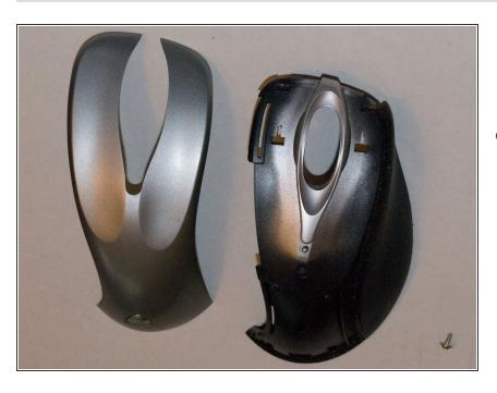
Remove the screw from the cover with a #1 Phillips. Unclip the two fins from the plate by lifting up on each gently. Remove the silver plate by prying the cover striaght up.
